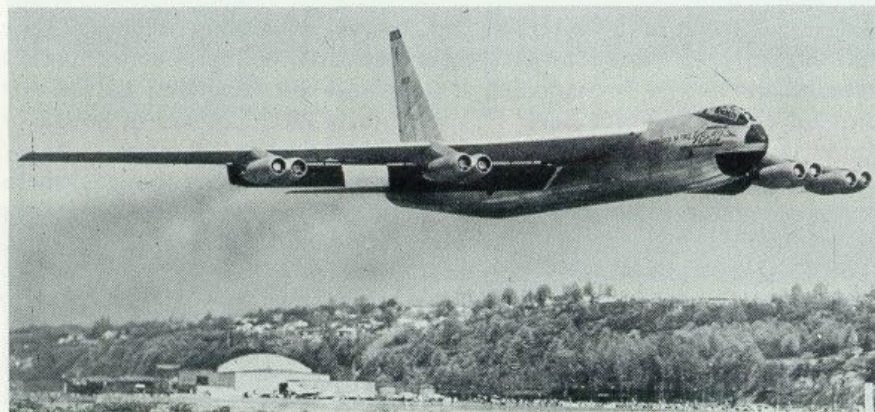
At the time of first flight, April 15, 1952, the four-unit landing gear of the YB-52 was a classified item. At Air Force request, the initially-released photos of the first flight had the landing gear touched out. Unretouched photo released later is shown for comparison. (Photos: Boeing)
