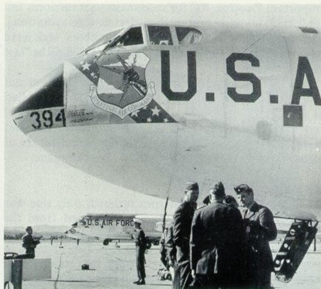
Outwardly, the B-52B was similar in appearance to the B-52A. This B-52B-35-BO (USAF: 53-394), with SAC emblem, white thermal-reflective paint and the 36-inch high "U.S. Air Force" lettering, is one of three B-52Bs that completed a non-stop flight around the world on January 18, 1957. Other two (here) are 53-397 and -398. (Photo: Boeing)
