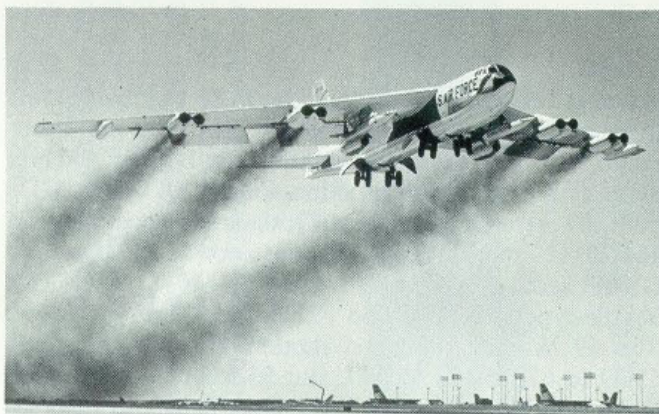
A B-52G with 700-gallon (U.S.) drop tanks being used by the Air Force to test electronic countermeasures pods that can be seen under the wings between the inboard and outboard nacelles. Note the double theodolite target markings fore and aft on the fuselage. (Photo: USAF via Boeing)
