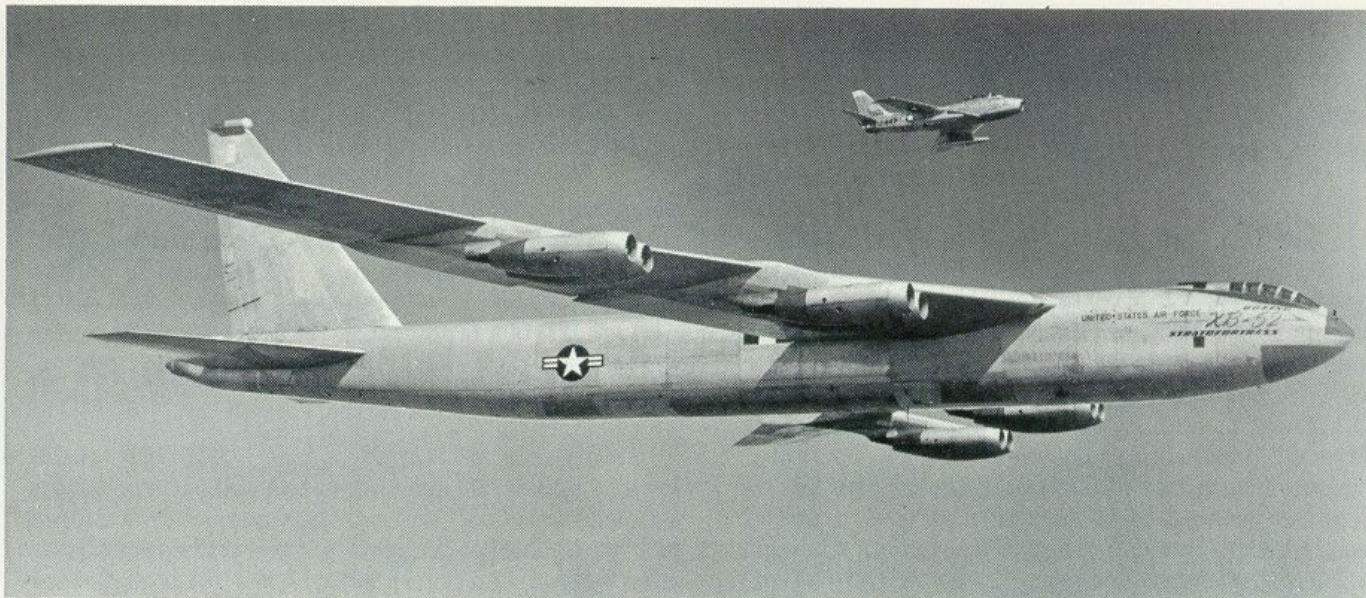
The prototype Boeing XB-52 (USAF serial number 49-230) on an early test flight accompanied by a North American F-86 Sabre "chase plane". The device at the top of the vertical fin is part of the test equipment. (Photo: Boeing)
