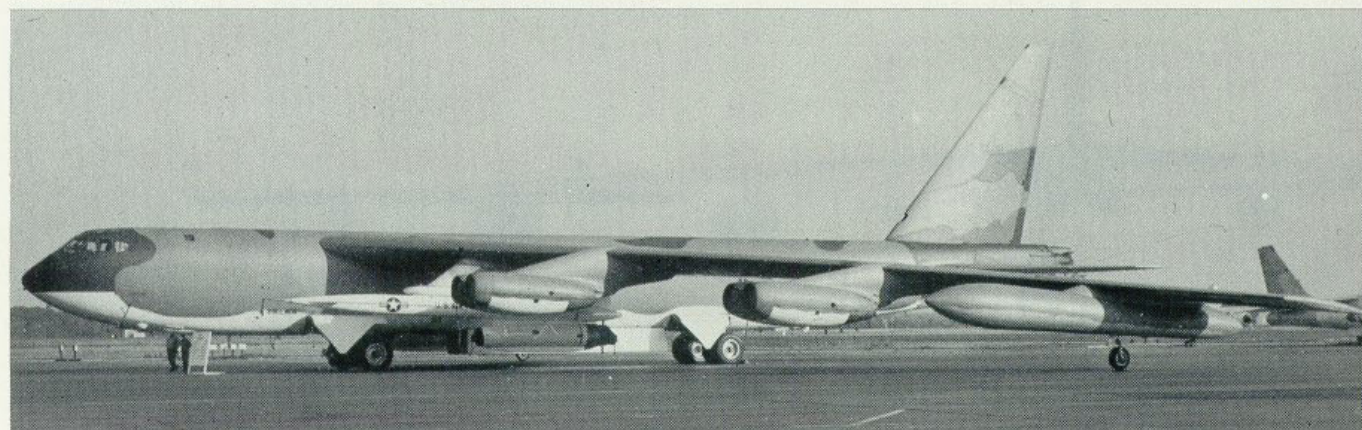
A Wichita-built B-52E (USAF: 56-701) with the standard camouflage scheme used on nuclear-weapons carriers; two-tone green and tan, with white undersides. Two white-painted AGM-28 Hound Dog missiles are carried. (Photo: author)
